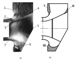
Figure 5 Reconstruction of the Westinghouse gas turbine compressor inlet duct: a) Flow structure at the flow passage of the Westinghouse gas turbine, b) Flow passage of the gas turbine with inserts-curves upon reconstruction
