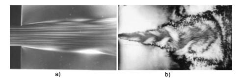
Figure 2 Visual diagnostics of flow structure: a) the laminar mode, b) the turbulent mode
