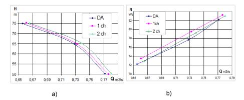
Figure 7 Results of blower modernization DA-210: a) the pressure characteristics P = f(Q), b) the power cost characteristics  $N_{el} = f(Q)$
