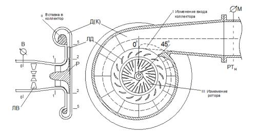
Figure 6 Drawing for reconstruction of blower DA-210
