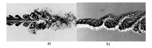
$\label{eq:Figure 1} Flow \ visualization, \ effluent \ in \ the \ flooded \ space: \ a) \ the \ smoke \ visualization, \ b) \ the \ spark \ method$
