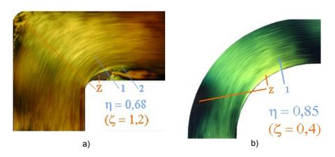
Figure 3 Flow structure in flow turn by 90°: a) "bend"  $\eta_D = 0,68$ , b) "lateral"  $\eta_D = 0,85$
